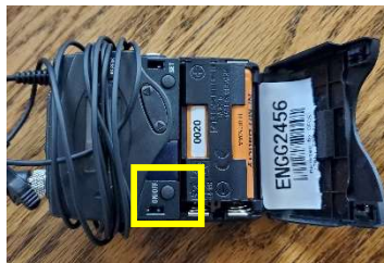
Flip open front of pack, press and hold power button to turn mic on/off.
