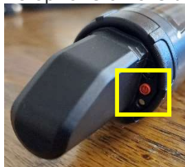
Press and hold power button to turn mic on/off.
