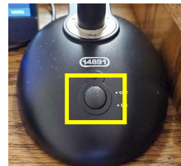
Press button to toggle podium mic on/off. Light will indicate power.
