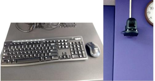
There is a wireless mouse and keyboard located that is connected to the PC. There is power switch located on the top right corner of the keyboard and the bottom of the mouse. Make sure these are on before you start your presentation.
